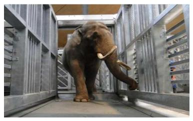
Zoo Zurich uses a tailormade weighing platform from METTLER TOLEDO to monitor their elephants' weight. The scale has already passed the crucial test, as all the animals have already been weighed. Despite this, the animals remain a little suspicious when the plate over the weighing cells moves a couple of millimeters.
